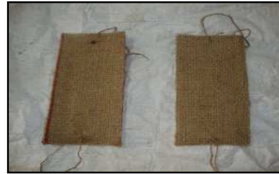
Photo 6: Jute samples ready for impregnation with bitumen
